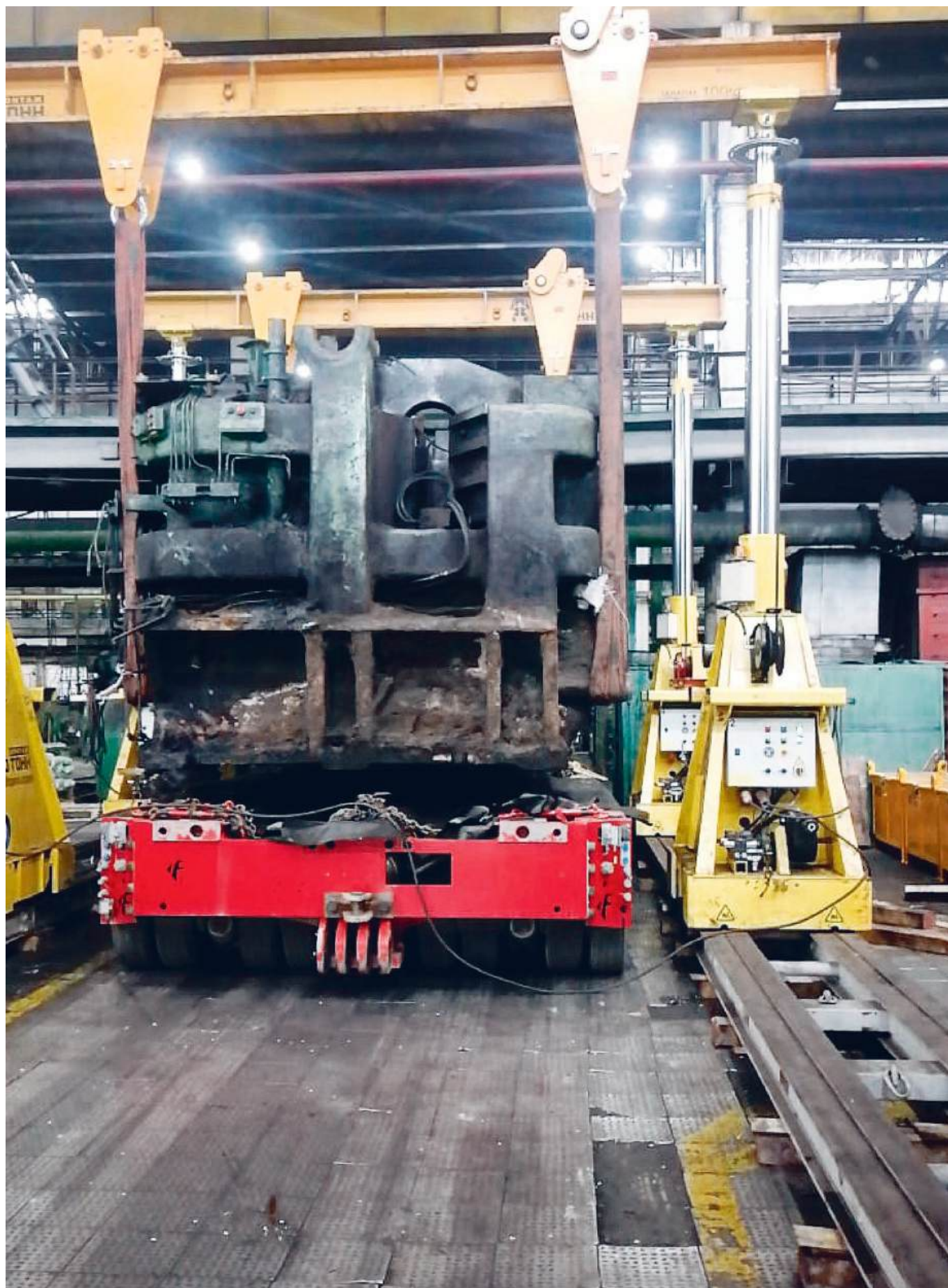
Automobile plant, Ulyanovsk city. Relocation of forge shop equipment.
